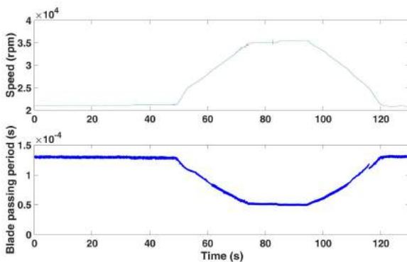
FIGURE 2: A typical run profile
