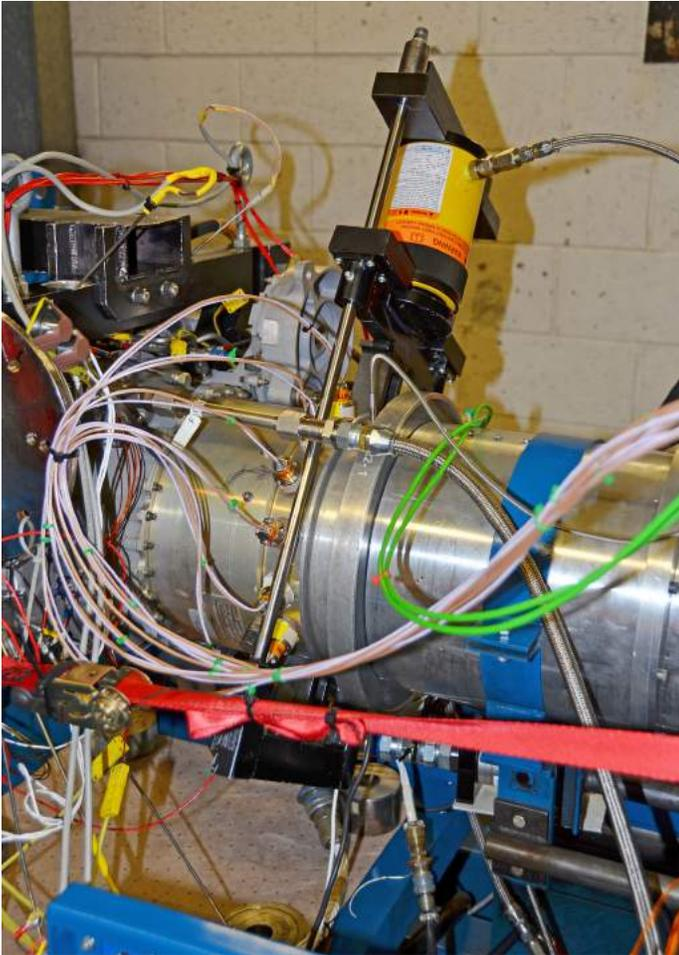
**FIGURE 3:** Hydraulic ram to squeeze the casing
