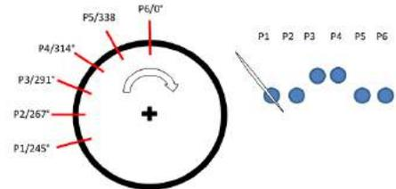
(c) Locations of the sensors on the engine
