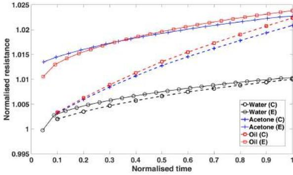
**FIGURE 5:** Comparison between CFD and Experimental data without contamination
