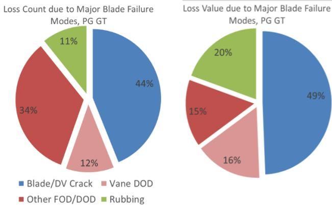
**Figure 3-1: Distribution of gas turbine loss by count and value, per major blade damage mechanisms**
