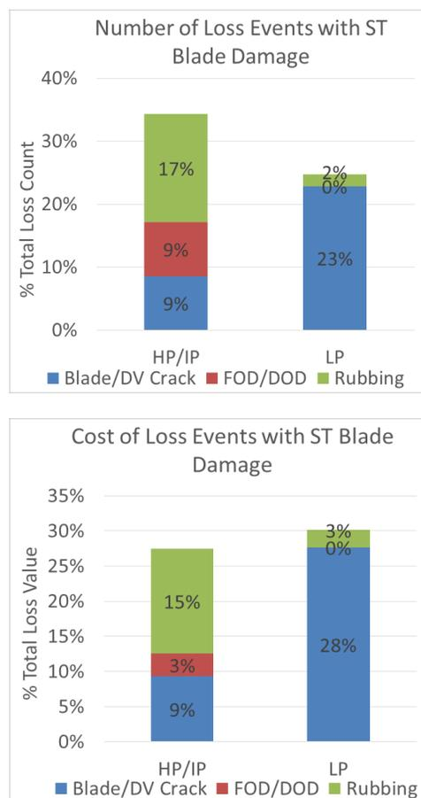
**Figure 3-7: Steam turbine loss with blade damage by count and value, per sections and damage mechanisms**
