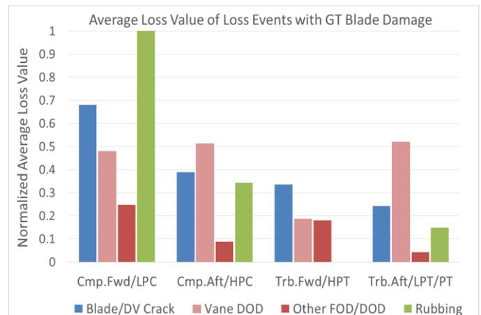
**Figure 3-4: Average value of gas turbine loss with blade damage per turbine sections and damage mechanisms**
