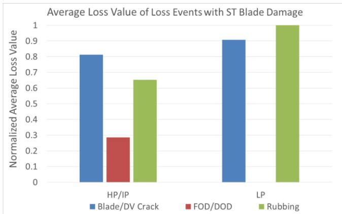
**Figure 3-8 Steam turbine loss with blade damage per sections and damage mechanisms**
