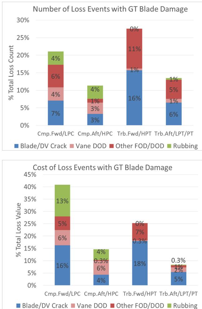
**Figure 3-3: Distribution of gas turbine loss with blade damage by count and value, per turbine sections and damage mechanisms**
