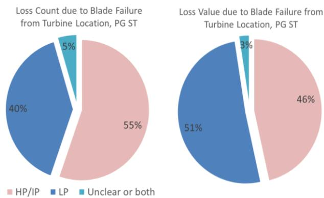
**Figure 3-6: Distribution of steam turbine loss by count and value, per blade damage locations**
