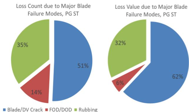
**Figure 3-5: Distribution of steam turbine loss by count and value, per blade damage mechanisms**
